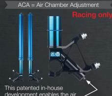
This patented in-house development enables the air chamber to be adjusted by means of a hexagon.
